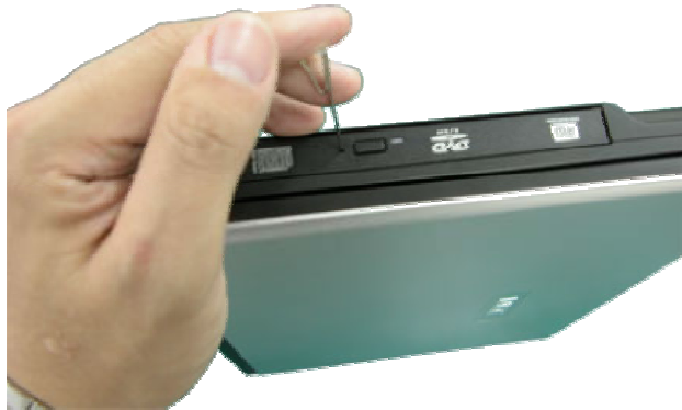
Fig. 5 Ejecting ODD tray
